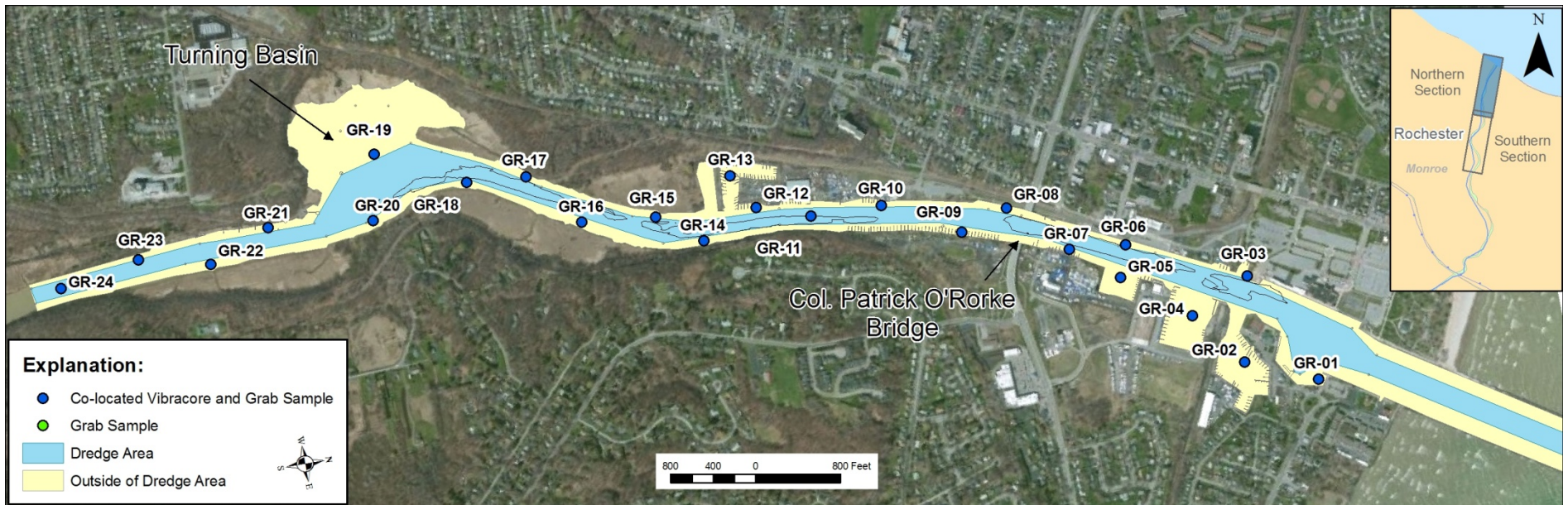
Figure 2-1a. Actual Sediment Sample Locations Adjacent to Dredged Navigation Channel and within Marinas
